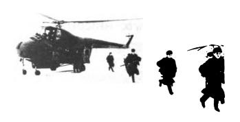
Figure 6-59. Mi-4 HOUND. A piston-engine single-rotor helicopter for light loads, the HOUND is being replaced by the Mi-8 HIP as the standard troop carrier.
